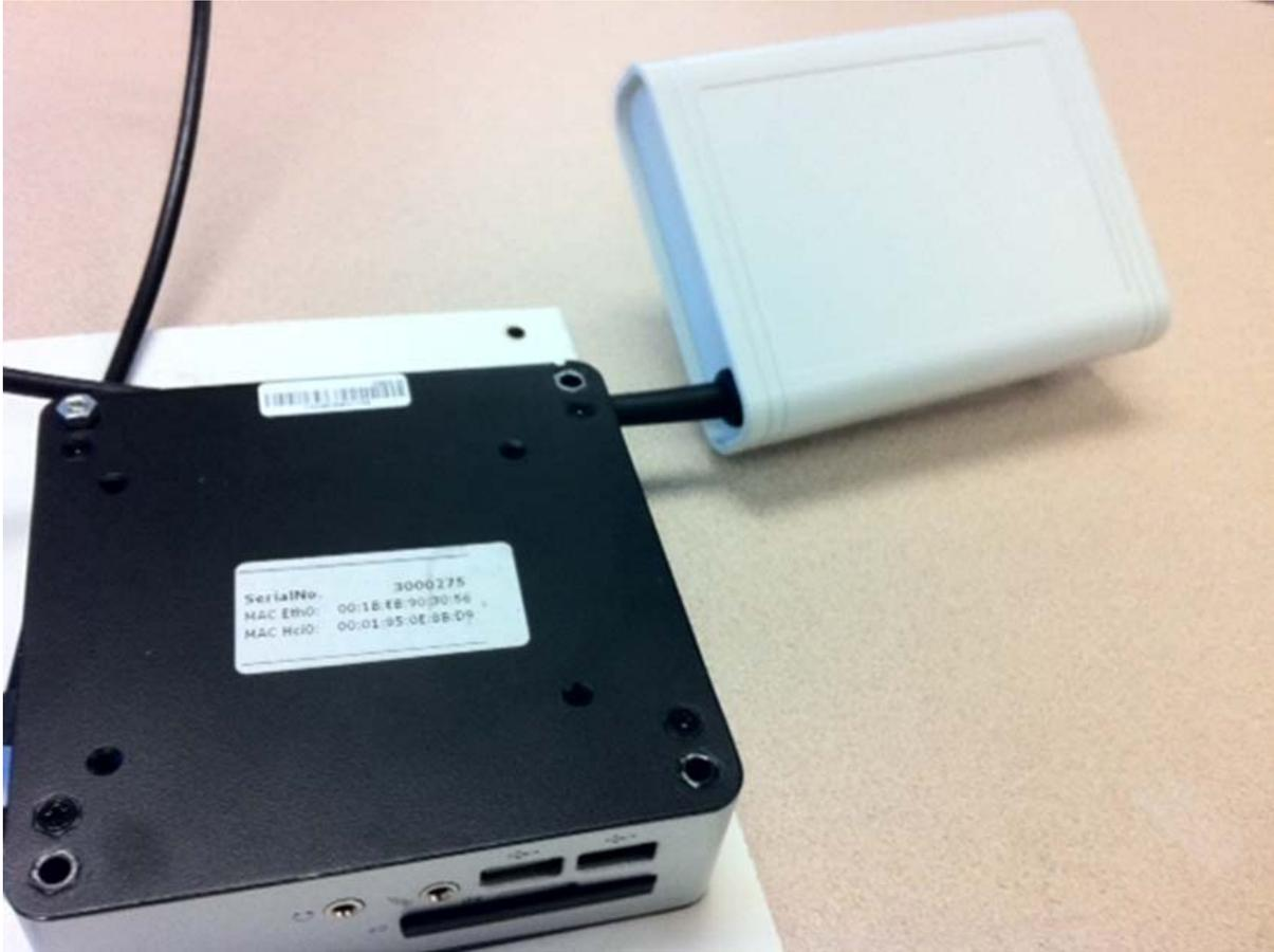
Bluetrace bluetooth scanner and directional antenna
